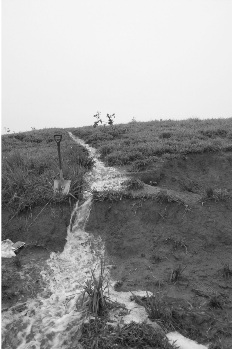
Figure 2. Photograph of the pasture hillslope as viewed from the overland flow sampling location, with runoff at the end of an 11-mm rainstorm (flow ~5 l/s). The lip is the sampling location for the HOF volume measurements and water sampling (marked HOF SL in Figure 1). The photo is taken facing northeast; the cattle trail conveying the water is marked CT1 in Figure 1
