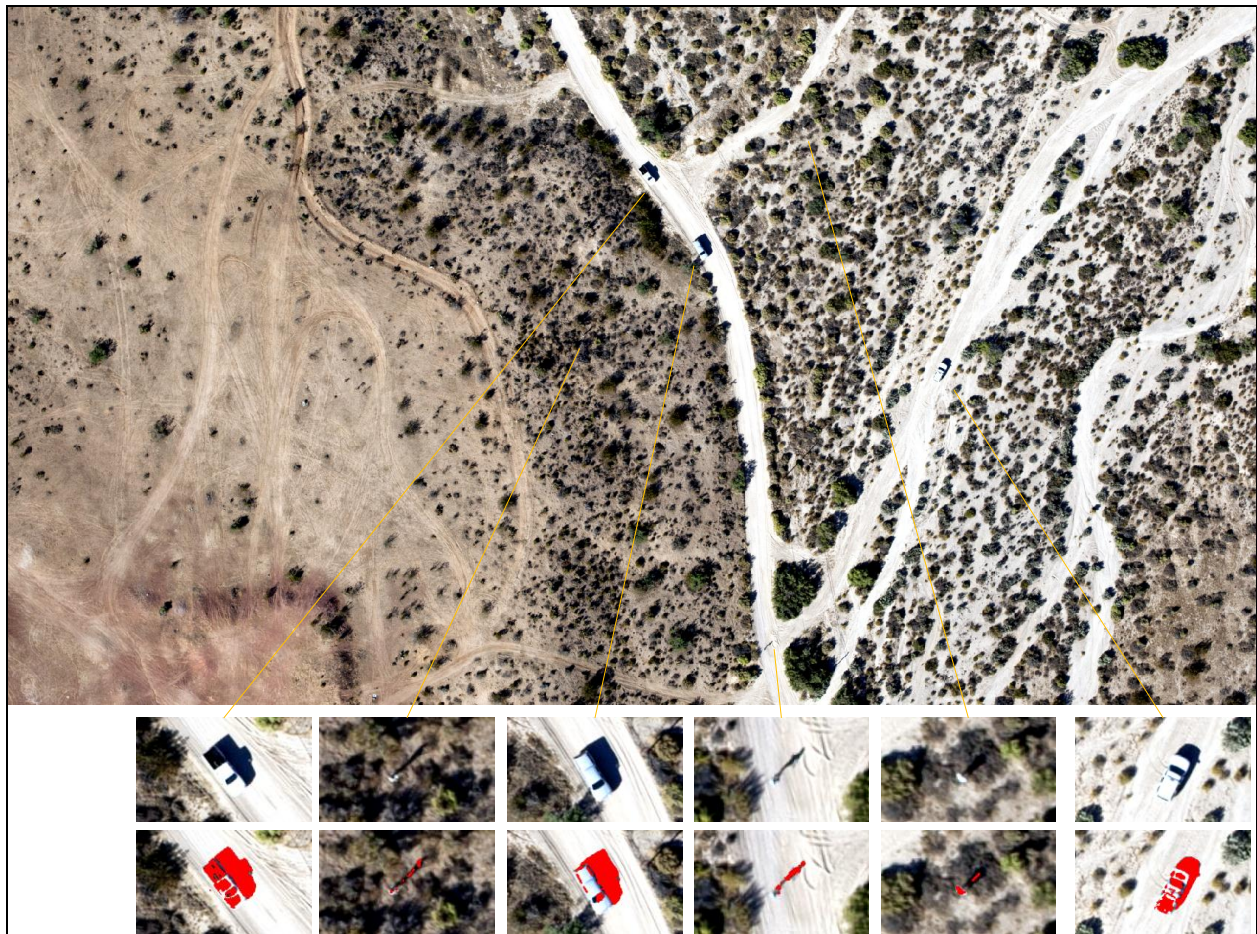
Figure 4. Image-based detection of people and vehicles moving within the U.S./Mexico border region. SDSU and Border Patrol personnel are detected as they move through a desert area (site 1) near Jacumba, CA. Red indicates detection of movement, as people or vehicles were not at the current location during the previous imaging passes. All people and moving vehicles were detected, with no false detection (commission error).
